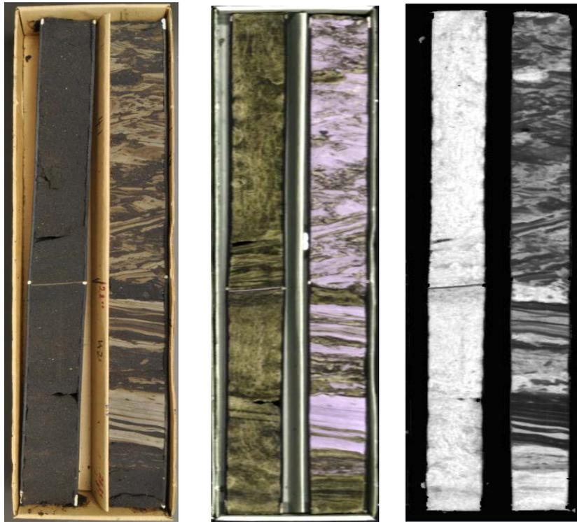
Figure 1: A dry core sample, from left to right: photograph, digital image (shortwave infrared) and greyscale TBC image. Despite the extensive devolatilization of the core, the greyscale image reveals coherent domains of variable bitumen saturation (black represents zones that are void of bitumen and white represents highest grade ore). Note that the mottled appearance of the bitumen saturated sandstone in the infrared image reveals a bioturbate texture otherwise not discernible.
