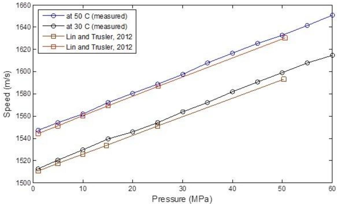
Figure 3: Speeds of sound in pure water at temperatures of 30° C and 50° C as a function of pressure are plotted along data from Lin and Trusler, 2012. The differences among them are due to the small variation in temperature and pressure (e.g., they measured at exact 50° C whereas our measurements were done at 50.5° C and also had pressure difference of ~0.1 MPa).
