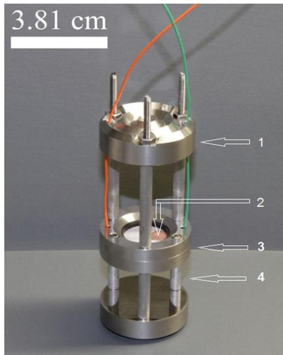
Figure 1: Image of ultrasonic pulse echo cell. 1. Stainless steel reflector, 2. PZT transducer, 3. PZT holder-transducer sandwiched between two stainless steel disc (Delrin used in between for insulating PZT with steel), and 4. Three rods (spacers).
