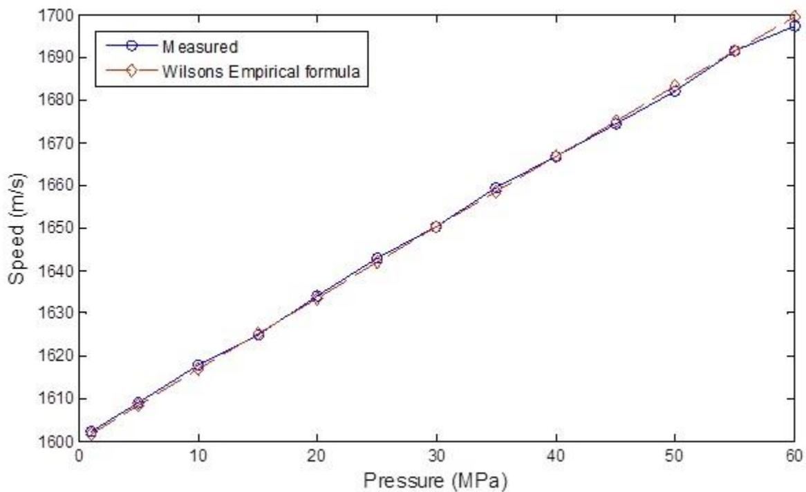
Figure 4: Speeds of sound in water with  $10^5$  ppm salinity at 30° C as a function of pressure. The data is plotted along with speeds from Wilson's empirical formula for sea water (Wilson, 1960).
