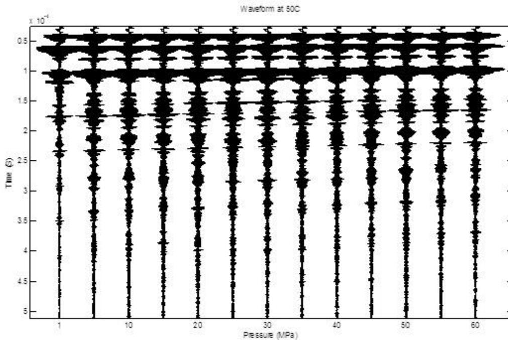
Figure 2: Waveforms of the echoes of the double reflectors method at pressures from 1 to 60 MPa and temperature of 50° C. The differences of onsets of first two echoes provide the transit time.
