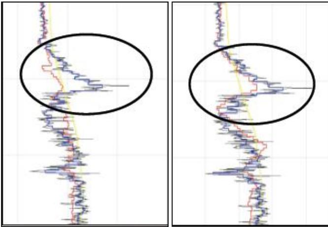
Figure 6: Conventional (left) and variable depth streamer (right) post-stack inversion P-impedance ( $I_p$ ) results plotted at the blind well. The initial model is shown in yellow, the inversion results in red, the well log ( $I_p$ ) in black and an upscaled version in blue. Inversion of the broadband variable depth streamer data results in a better well tie, while the conventional result is trapped near to the initial  $I_p$  model.
