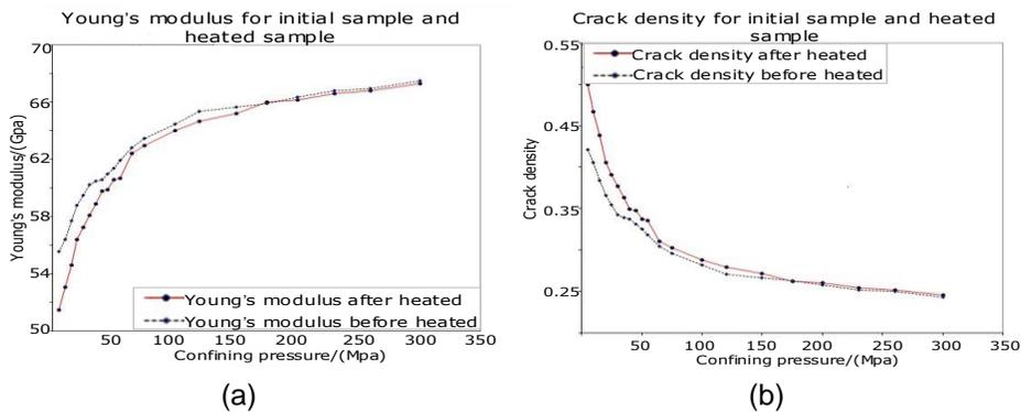
Figure 4 Modulus Comparison and Crack density comparison (a) Young's modulus for initial sample and heated sample (b) Crack density for initial sample and heated sample
