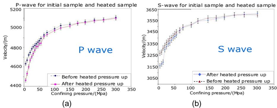
Figure 3 Wave velocity comparison (a) P wave velocity for initial sample and heated sample. (b) S wave velocity for initial sample and heated sample
