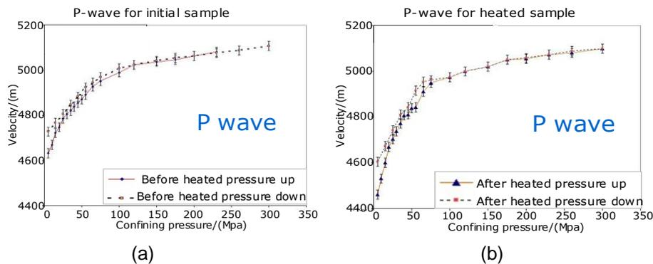
Figure 2. Wave velocity with pressure change. (a) P wave velocity for initial sample. (b) P wave velocity for heated sample.
