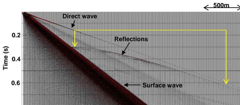
Figure 2: A vertical component synthetic seismogram with a strong surface wave, direct wave and reflections (relative true amplitudes). The optimum offsets window for shallow high density targets is indicated by yellow arrows and is 600-2000m.
