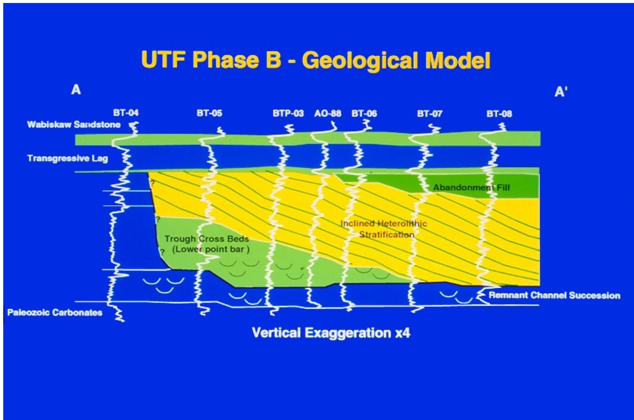
Figure 2. Geological model proposed for the B2 well pair at the UTF Phase B pilot (Strobl et al., 1997)
