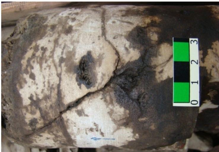
Figure 3. Core photography of heavily oil stained dolomite reservoir rock with excellent vuggy and fracture porosity from the upper member of the Birdbear Formation at Well Nuvista Mackin 111/12-04-039-27W3.
