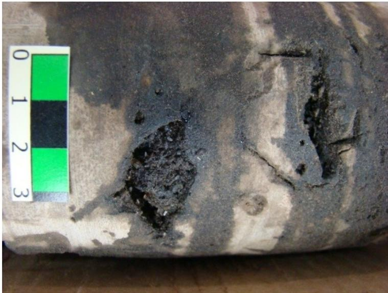
Figure 2. Core photograph of heavy oil dolostone reservoir rock from the upper member of the Birdbear Formation at Rife et al Eureka 131/14-02-032-23W3. Note the intensity of oil stain and the excellent interparticle, fracture and vuggy porosities that are partially filled by oil-stained calcite crystals.
