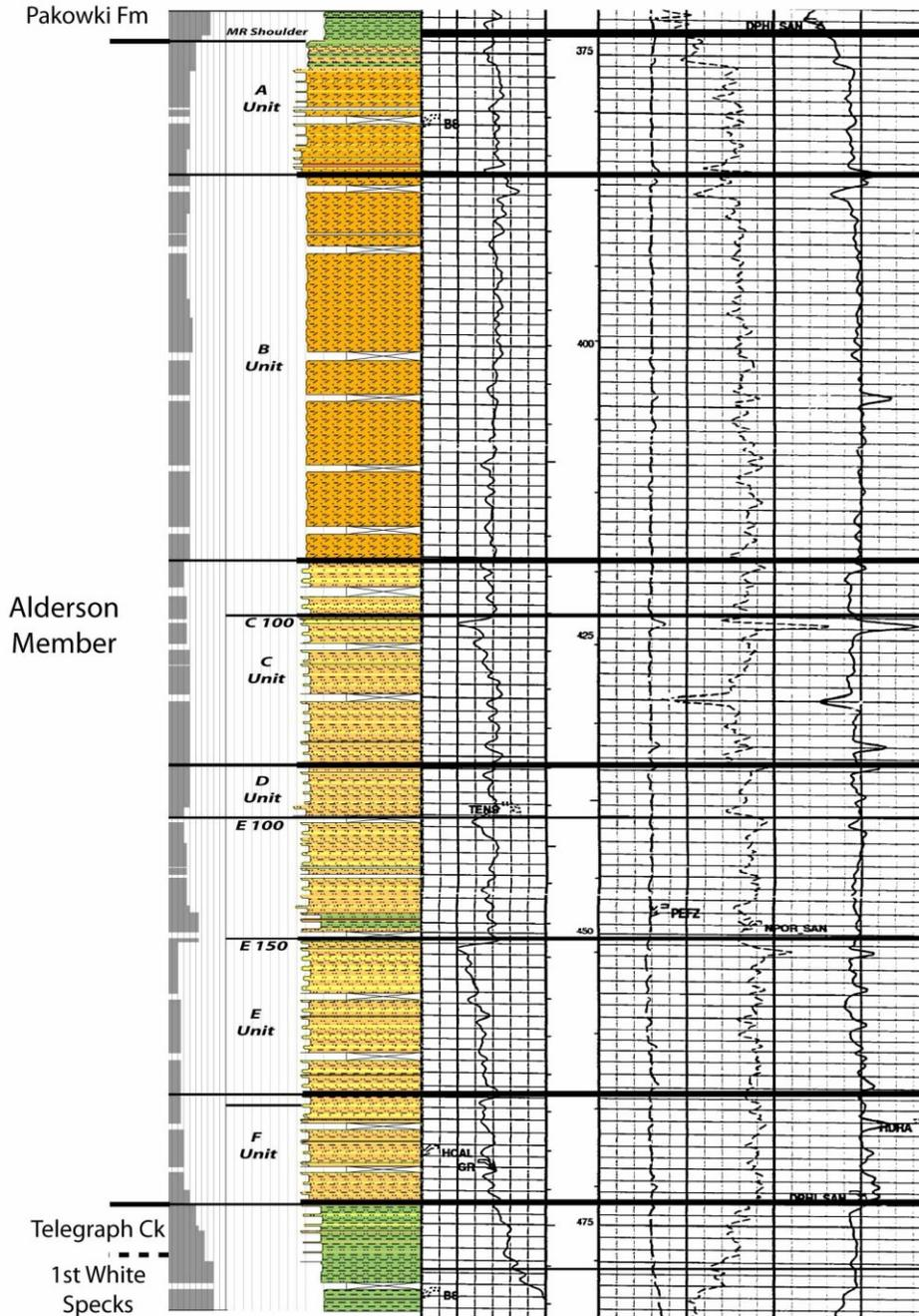
Lithological description of Nexen Medhat 6-31-14-1w4 with gamma - neutron/density log
