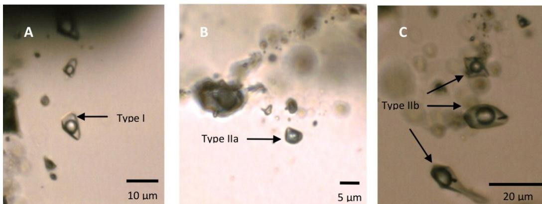
Figure 3. A) Type-I, aqueous fluid inclusions in quartz associated with primary ore; B) Type-IIa, aqueo-carbonic inclusions in quartz associated with secondary ore; C) Type-IIb, secondary aqueo-carbonic inclusion with opaque daughter mineral in quartz associated with primary ore. All in transmitted plane polarized light.
