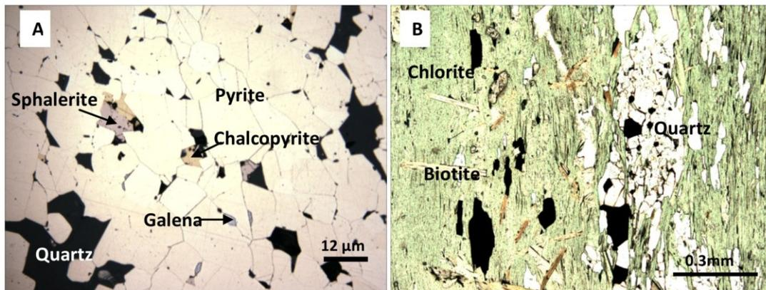
Figure 2. A) Photomicrograph of sulphide ore minerals and associated quartz in primary massive ore; reflected light; B) Photomicrograph of sulphide minerals and quartz veinlets that have been stretched parallel to schistosity; transmitted plane polarized light.
