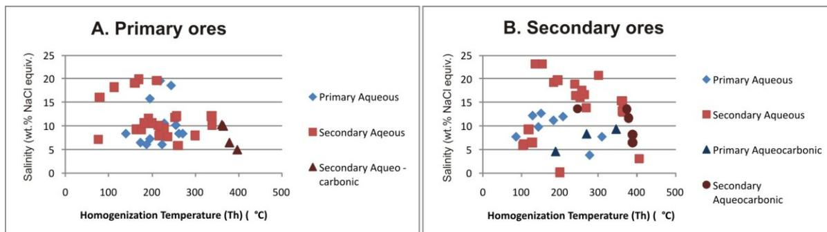
Figure 4. Salinity-homogenization temperature correlation diagrams for fluid inclusions in primary (A) and secondary ore (B).
