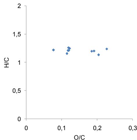
Fig. 2. The elemental analysis of the domanik kerogen samples on the Van Krevelen diagram.
