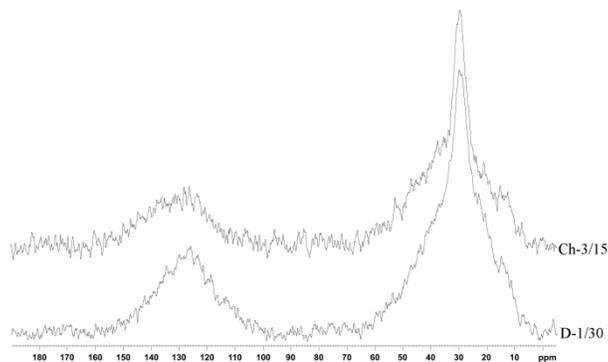
Fig. 3.  $^{13}\text{C}$  NMR spectra of Domanik kerogen from Chut (Ch-3/15) and Domanik (D-1/30) rivers (Bushnev et al., 2010).
