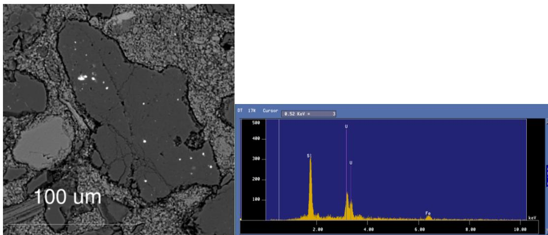
Figure 3: a) Microprobe back-scattered image of uranium-bearing quartz grain from Willow Creek Formation siltstones; b) Representative EDX spectrum confirming presence of U in inclusions
