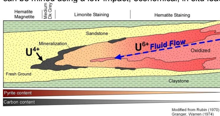
Figure 1. Roll-front deposit model.
