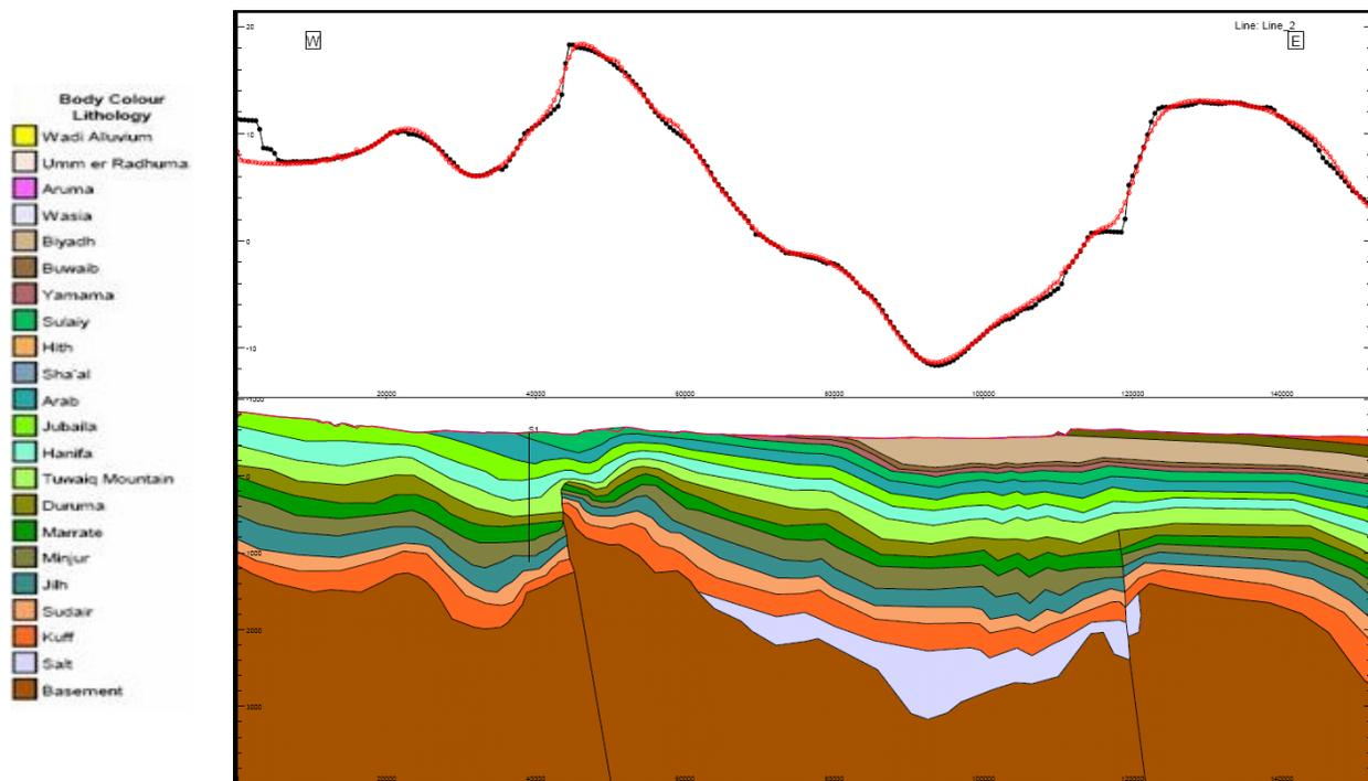
Figure 3 Gravity model for profile no. 3 shown the salt layer.
