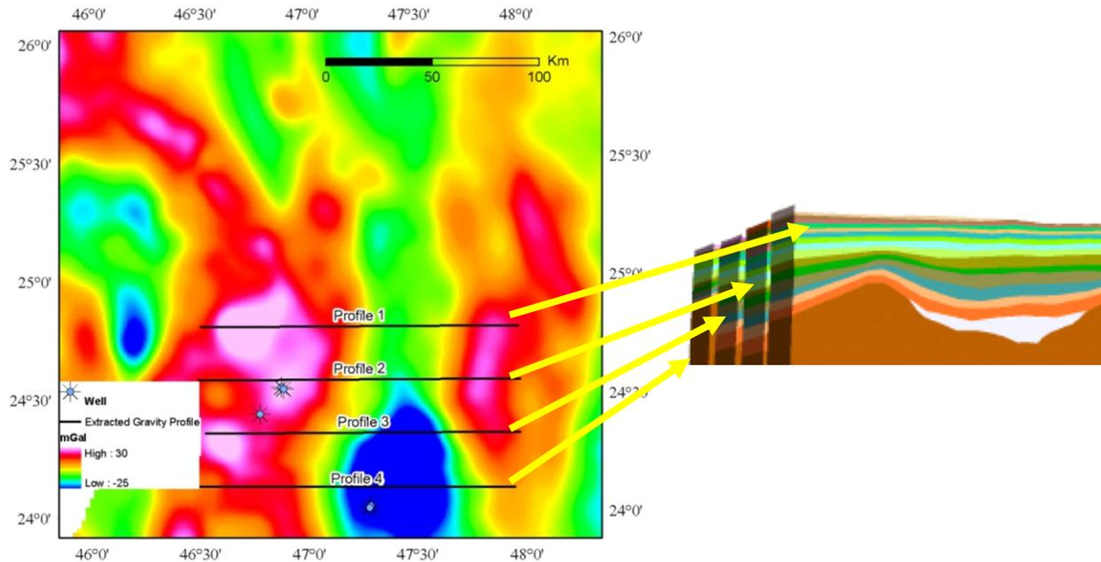
**Figure 2 Decompensative gravity anomaly map shown location of wells and the extracted gravity profiles used for 3D Modelling.**
