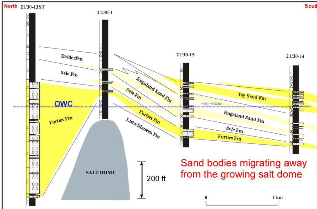
Fig. 3 North-South cross-section through the Gannet F Field
