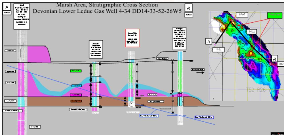
Figure 2: Stratigraphic cross section illustrating Ireton and reef thickness variation over the 4 wells drilled in the Marsh area
