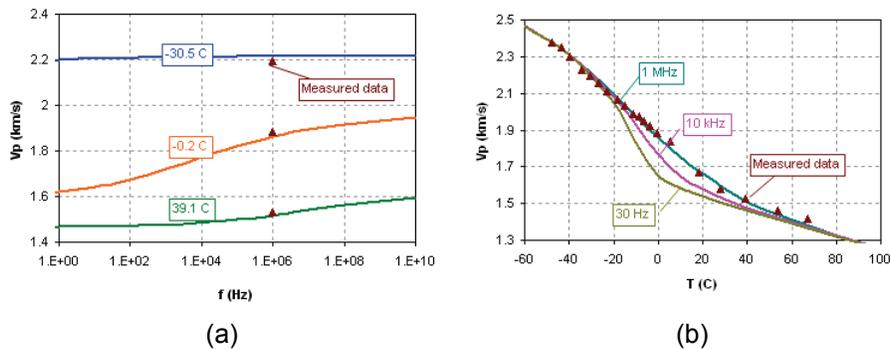
Figure 5: Estimated P velocity vs. frequency for a heavy oil with API = 9.38.
