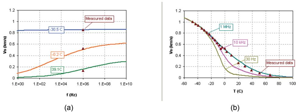
Figure 4: HN model for S-wave velocity applied on a heavy oil with API = 9.38.
