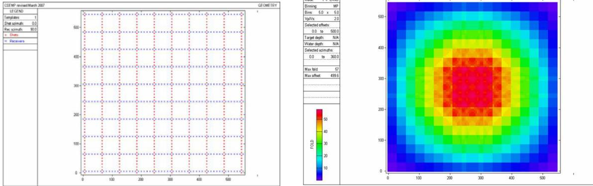
Figure 2: On the left is the layout design for the vertical component 3D baseline 3D survey. Receiver lines run east-west and source lines run north-south. On the right is the expected fold for the PP survey
