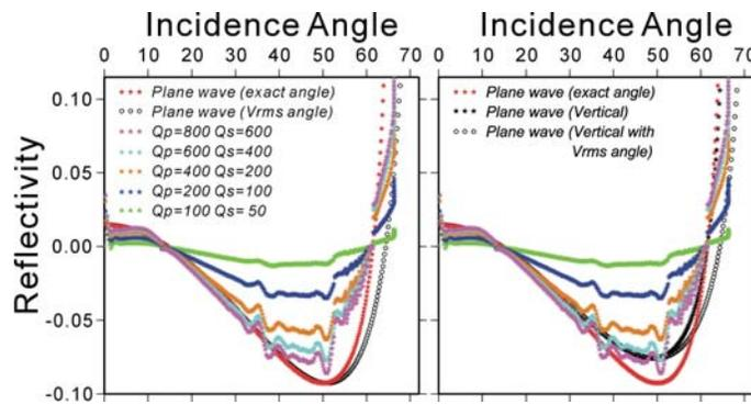
Figure 3: Scaled spherical-wave (numerical) reflection coefficients with constant  $Q_p$  and  $Q_s$  for top of layer 6 layers (Table 1). *Plane wave* denotes the same reflectivities calculated from Zoeppritz equation as in Figure 1.
