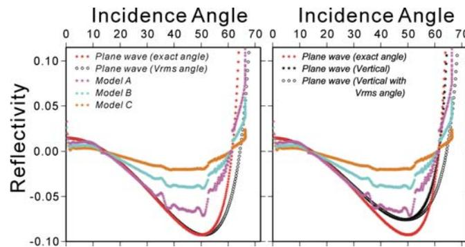
Figure 4: Scaled spherical wave reflection coefficients with varied  $Q_p$  and  $Q_s$  for top of layer 6 layers (Table 1). Quality parameters are set as follows:  $Q_p = (V_p / \text{Const})^2$ ,  $Q_s = 4Q_p / 3(V_s / V_p)^2$  (Udias, 1999), where Const equals 200, 150 and 101.5 respectively in Models A, B and C. *Plane wave* denotes the same reflectivities calculated from the Zoeppritz equation as in Figure 1.
