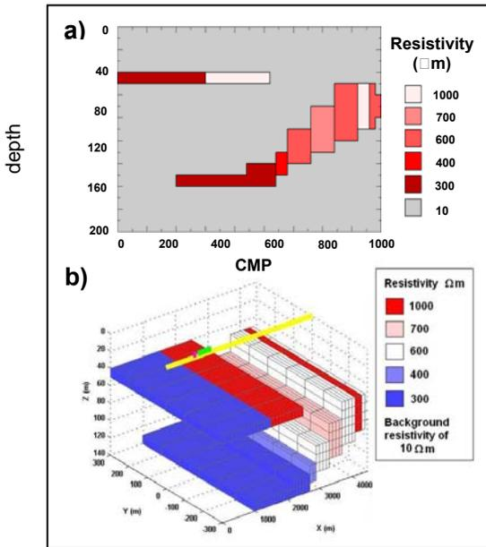
Figure 7: Cross-section and 3D view of test model
