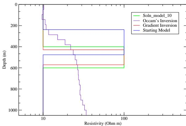
Figure 5: A 3-layer test model with a resistive layer
