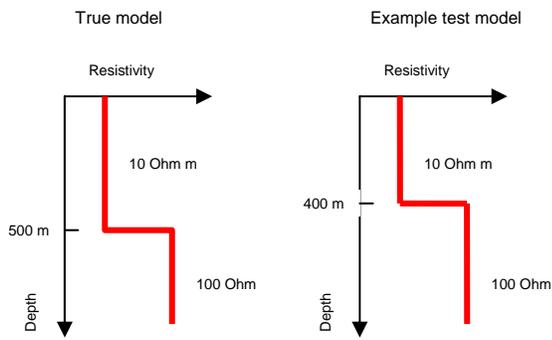
Figure 3: Synthetic model and example test model
