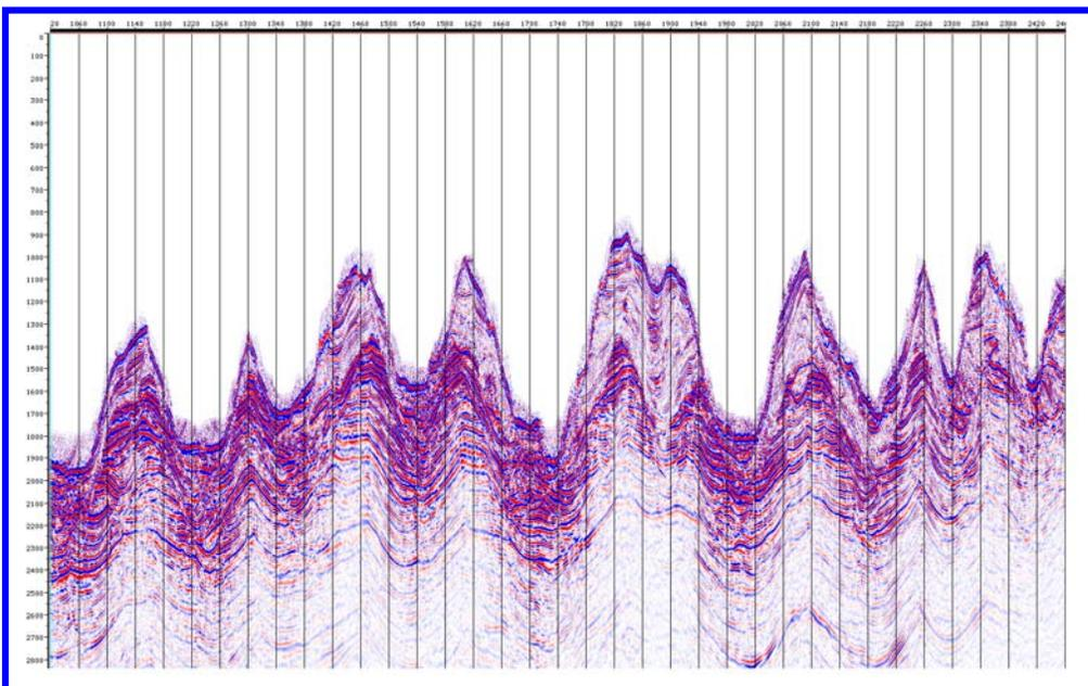
Figure 2. This crossline section from the migrated seismic block illustrates the complexity and roughness of the sea floor from this Brazilian dataset processed with 3D SRMM. It is a submarine canyon environment where the bathymetry varies from 200 to 2000 meter depth inline.
