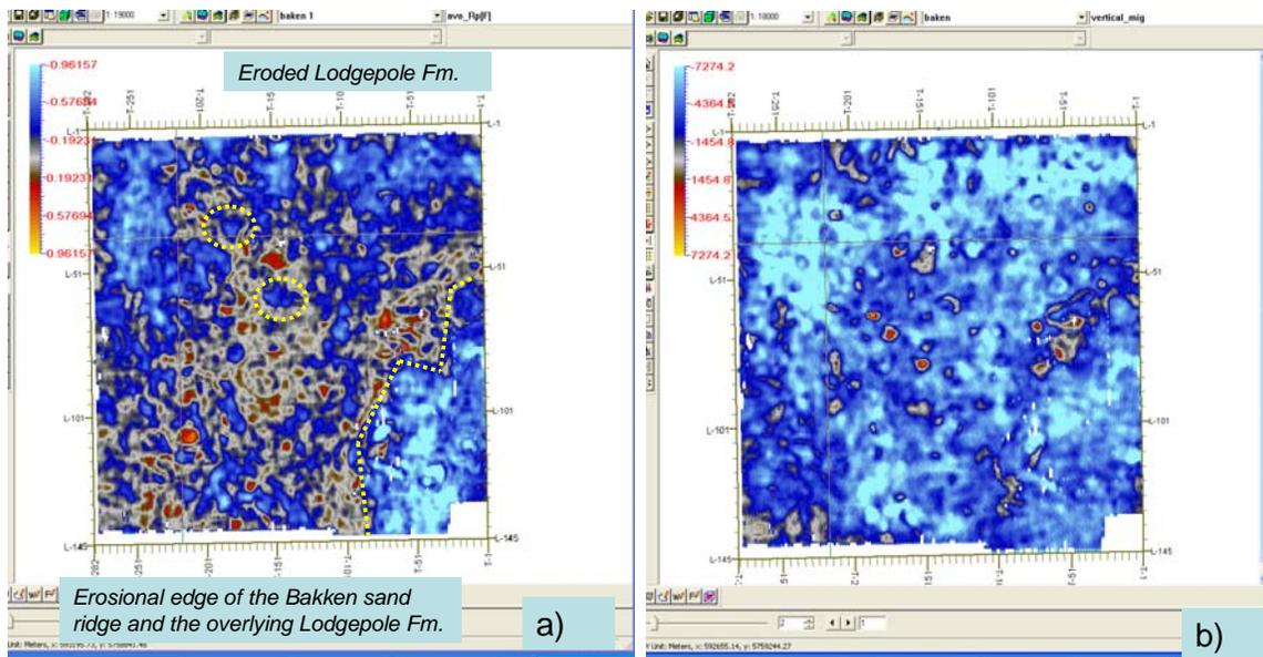
Figure 3: Horizon slice of the (a) AVO Rp and (b) Migration at Bakken+2ms
