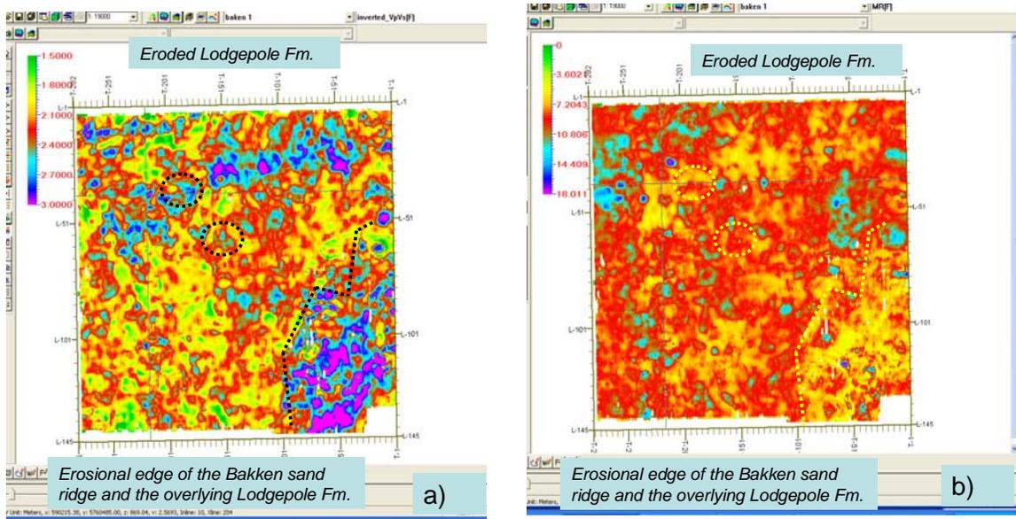
Figure 4: Horizon slice of the (a) Vp/Vs and (b) Mu-Rho at Bakken+2ms
