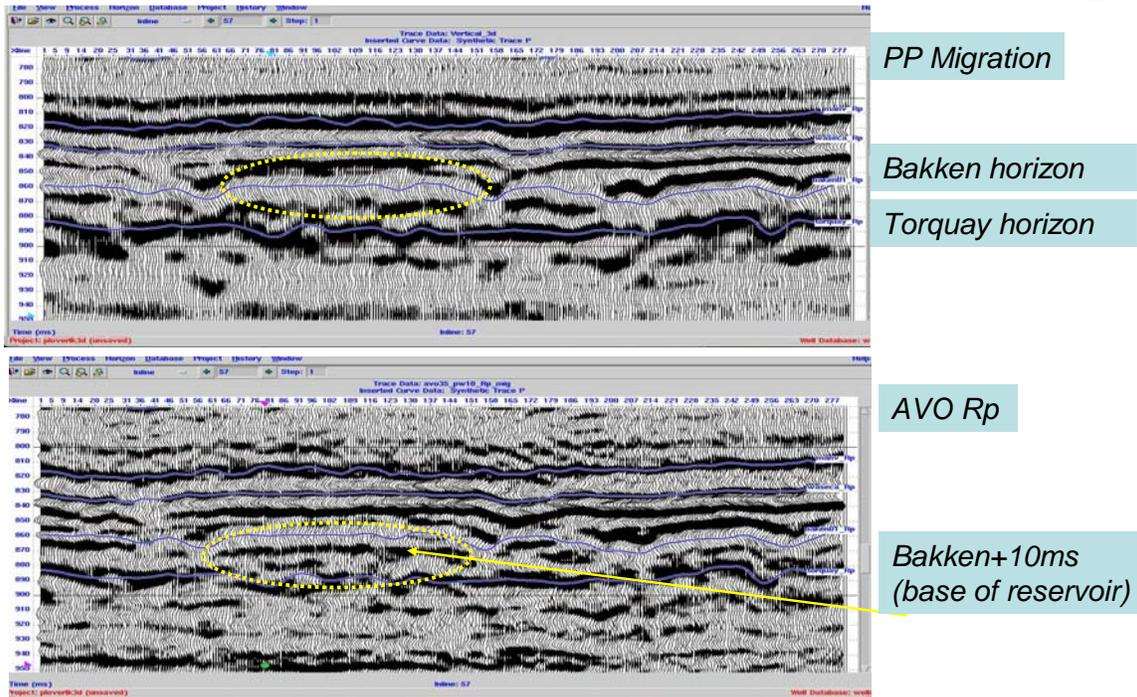
Figure 2: Comparison between PP-migration (top) and AVO Rp (bottom) showing higher resolution on the AVO Rp.
