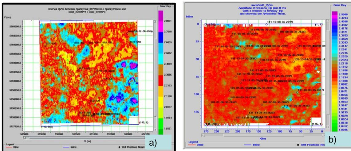
Figure 5: (a) Average Vp/Vs for interval Sparky-Torquay (Lines, et al., 2005) and (b) average Vp/Vs for interval Waseca-Torquay from simultaneous inversion
