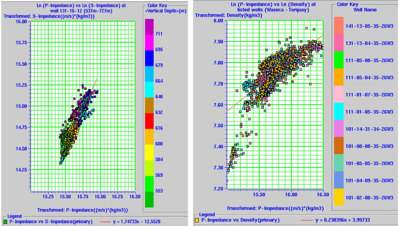
**Figure 1: left: relationship between ln(Zp) and ln(Zs) based on one dipole well:  $\ln(Zs)=1.74*\ln(Zp)-12.55$ ;
