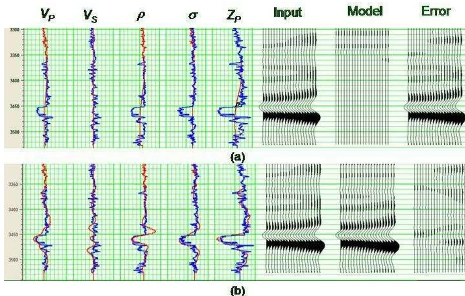
Figure 2. The results of inverting a gas sand model, where (a) shows the initial model before inversion, and (b) shows the results after inversion. In both plots, the original well log curves are in blue and the final estimated curves from the inversion are in red. The seismic gathers on the right hand side of the plot show, from left to right, the input model, the inverted result, and the difference between the input and inverted results.
