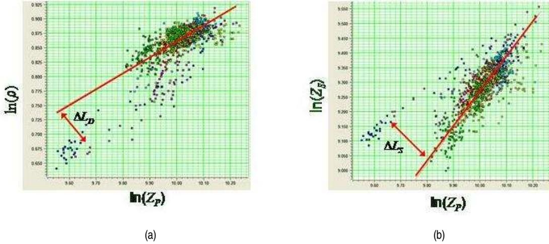
Figure 1. Crossplots of (a)  $\ln(Z_D)$  vs  $\ln(Z_P)$  and (b)  $\ln(Z_S)$  vs  $\ln(Z_P)$  where, in both cases, a best straight line fit has been added. The deviations away from this straight line,  $\Delta L_D$  and  $\Delta L_S$ , are the desired fluid anomalies.
