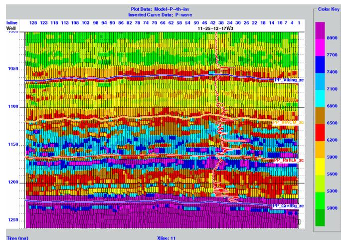
FIG. 2. Results of the model-based P-impedance inversion
