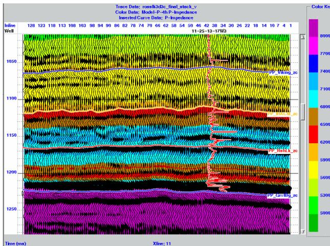
FIG. 1. The P-impedance model with P-impedance log inserted.
