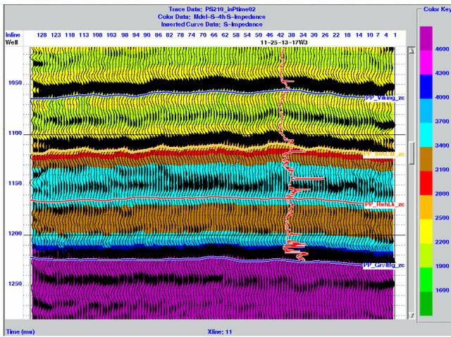
FIG. 4. The S-impedance background model.
