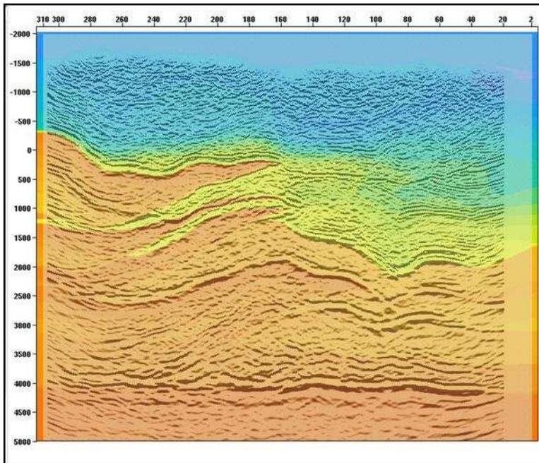
Figure 1: PreSDM Inline 120 with final velocity model overlay
