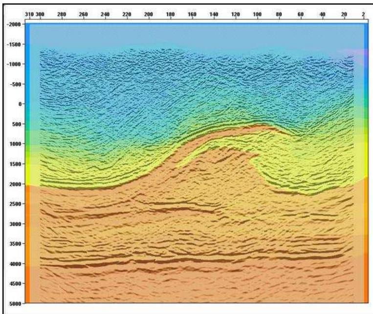
Figure 2: PreSDM Inline 320 with final velocity model overlay
