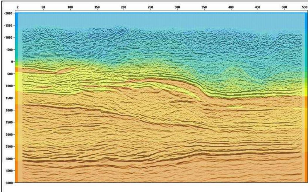
Figure 3: PreSDM Crossline 160 with final velocity model overlay
