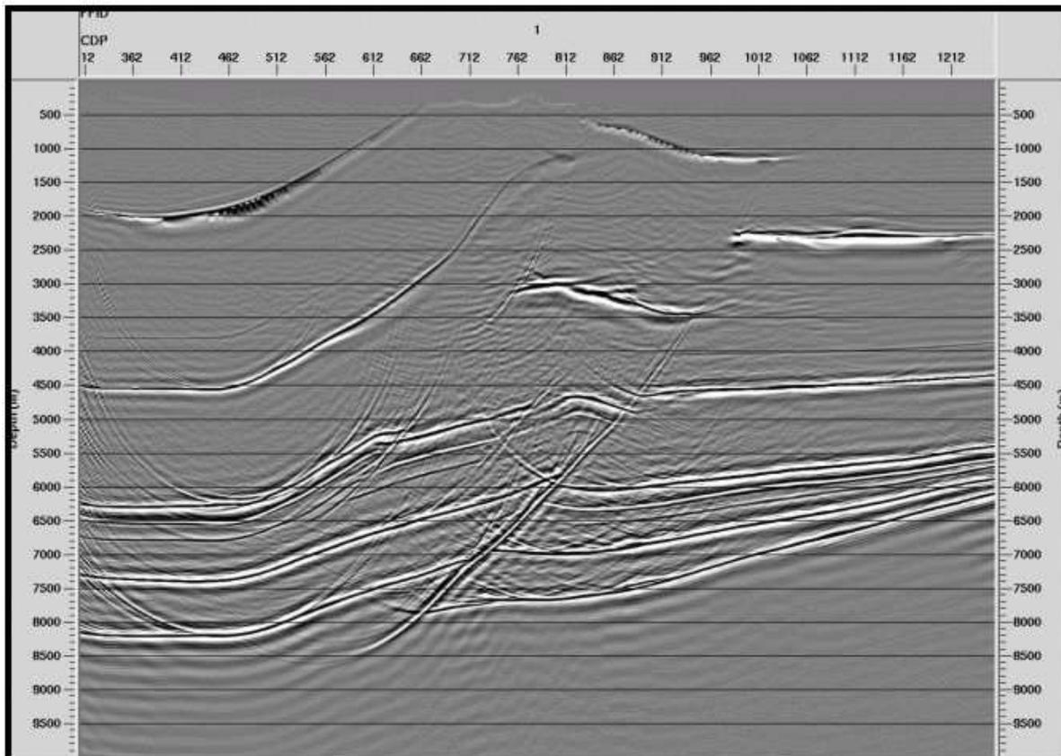
Fig. 3 Prestack FD depth migrated image of the model shown in Figure 2.
