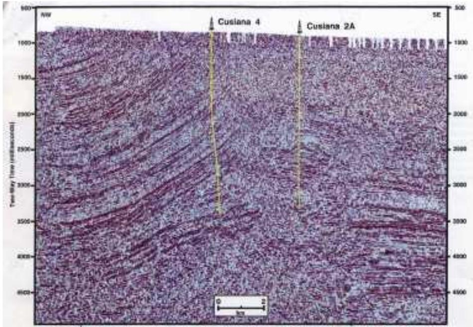
Fig 1: Seismic line T-1 across Cusiana oilfield with F-D prestack time migration
