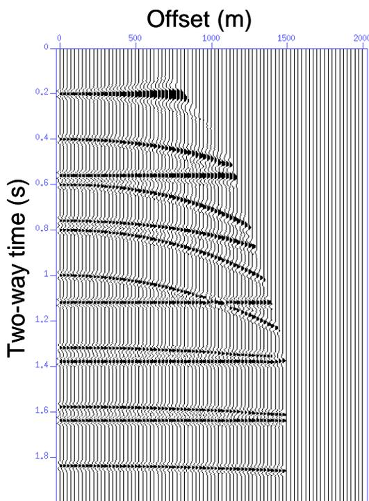
Figure 1 An NMO-corrected muted synthetic CMP data.
