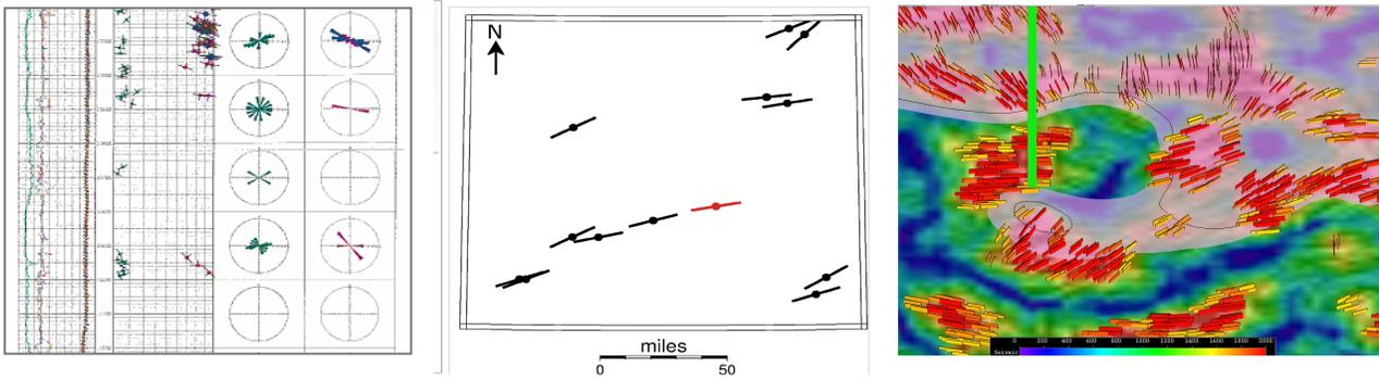
Figure 1: FMI log interpretation (left); regional stress map - WSM (middle); fracture density and direction (right) estimated from the AVAZ analysis around the location of one of the most prolific wells in the field (6 mmcf/day). Note the horizontal well path direction, a consistent E-W fracture direction is observed, and this is in agreement with FMI interpretation at the well location and the regional stress trend (Reinecker et al.).
