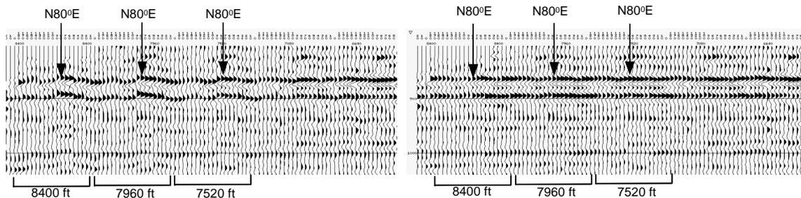
Figure 2. Azimuth-offset sorted NMO super-gather centered on the well location. Right: Note the variable travel time: minimum travel observed at N80°E orientation. Left: The same gather flattened. Note the larger amplitudes at the same direction. This is in agreement with AVAZ, FMI (at the well location) and WSM data that show the regional trend (Figure 1).
