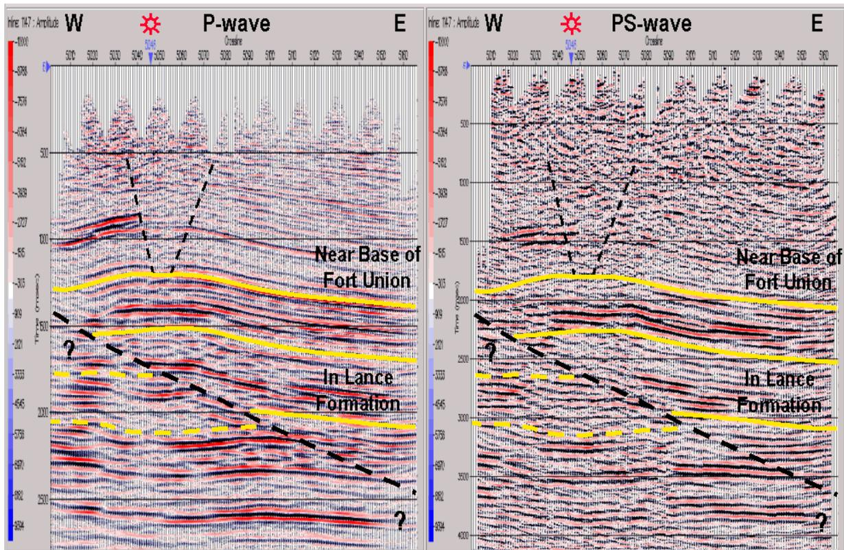
**Figure 1.** P-wave interpretation over the Pinedale anticline where production occurs in Cretaceous tight gas sands in the Lance formation. Note that the PS-wave section, compressed in time compared to the P-wave by a  $V_p/V_s$  factor of two, agrees very well with the P-wave interpretation.
