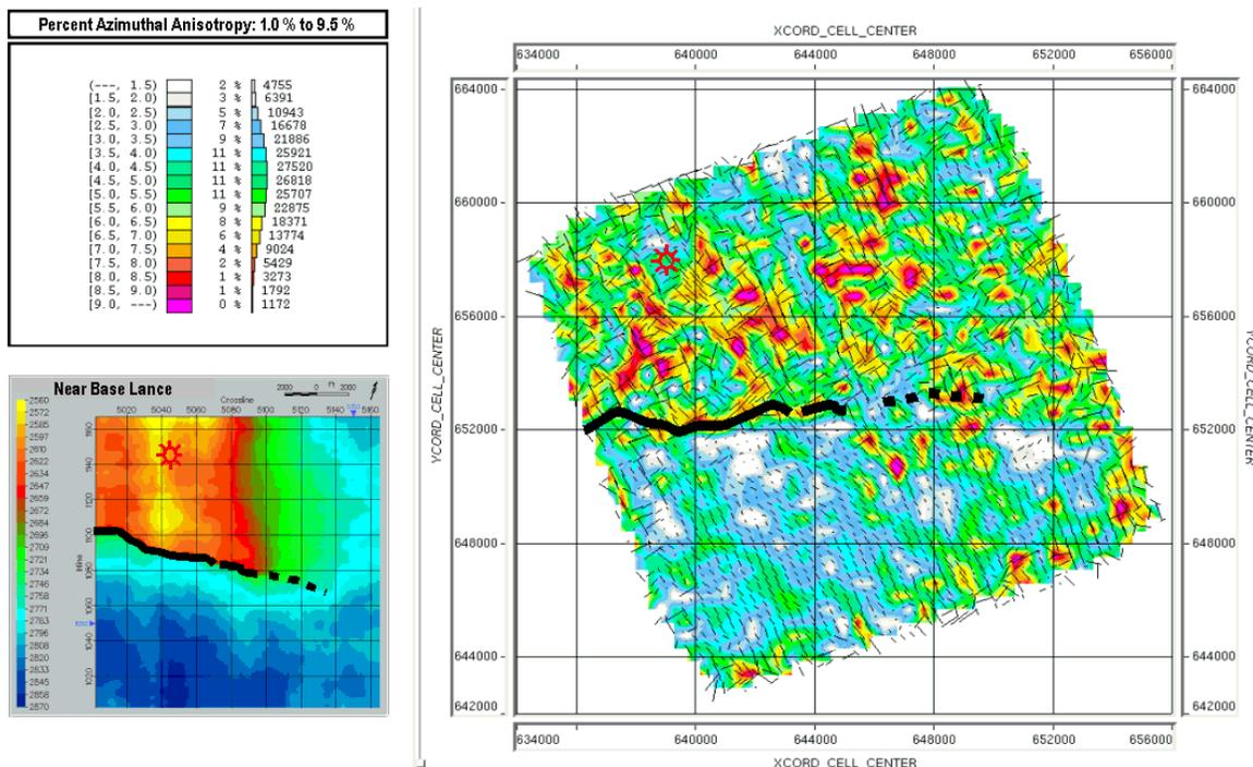
**Figure 3.** Azimuthal anisotropy analysis (right) over the target for near base of Lance isochron (left). Colors represent percent anisotropy (fracture intensity) from 1.0 to 9.5, which have a peak distribution at 4.5%. Again, note that more intense anisotropy occurs over the Pinedale anticline, but there are also high anisotropy areas further to the east.
