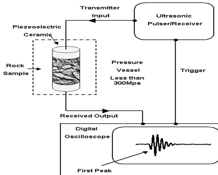
Figure 1. Schematic showing acoustic experiment setup
