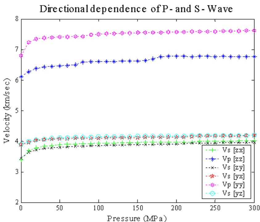
Figure 3. Measurements of Velocities and Anisotropy
