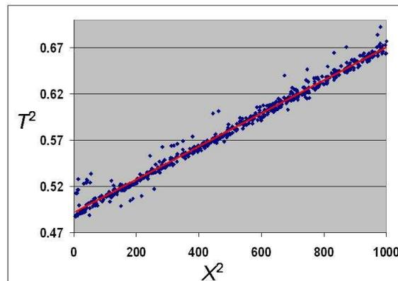
**Figure 1. Example of  $T^2$ - $X^2$  plot obtained from computing differential time shifts for a reflection event at 0.5s Two-Way-Time. The outliers are easily defined by statistical analysis and removed before the final fitting.**
