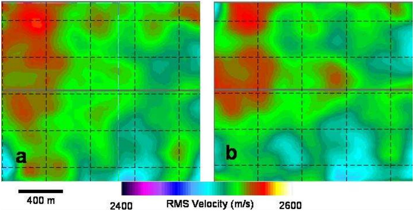
Figure 4. Map view of velocity field computed from 2 3-D surveys shot 1 year apart. The time slice was taken from above the reservoir, so no changes are expected. The two datasets were processed independently (independent statics solutions, deconvolution and gain), with only CMP-consistent matching to allow for comparison of equivalent time slices. The maximum difference is ~20 m/s, with most differences being less than 10 m/s.
