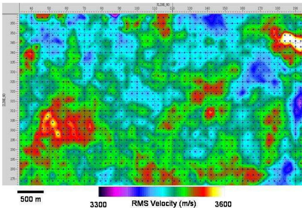
Figure 2. Time slice of velocities computed using the automated traveltime inversion. No smoothing has been applied and each blue dot represents an analysis location. No information is shared between analysis locations which are treated independently for the velocity inversion.
