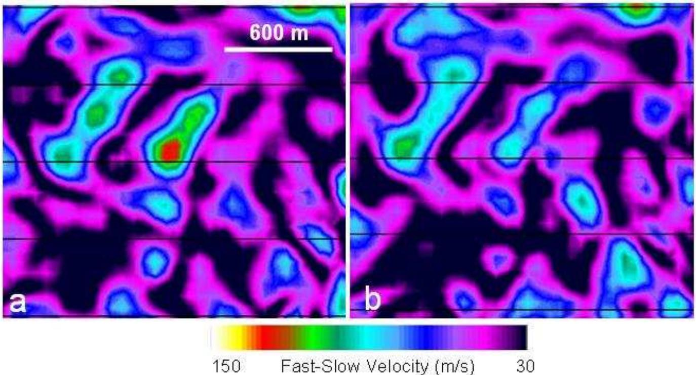
Figure 5. Azimuthal velocity anisotropy computed from the same two surveys used in Figure 4, again with independent processing. A smaller area is shown than in Figure 4 because of the wide-azimuth requirement for azimuthal velocity inversion.
