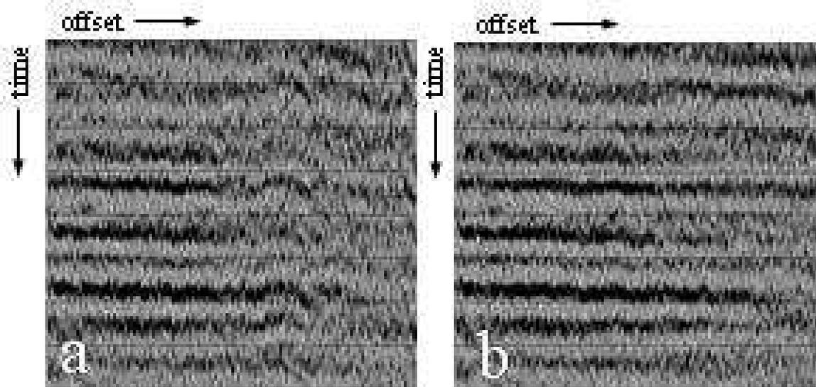
Figure 3. Example of a wide-azimuth CMP sorted as a function of offset (azimuths mixed) after processing which includes refraction and two passes of residual statics. a) best isotropic NMO correction and b) azimuthal NMO correction. The apparent anisotropy was found to be about 4% and dips in the area are less than  $3^\circ$ , which could account for only 0.3% of the apparent anisotropy.
