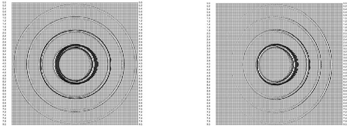
Figure 3: Time slices of migration impulse response at 600 ms from simple VTI (left) and TTI (right) models.
