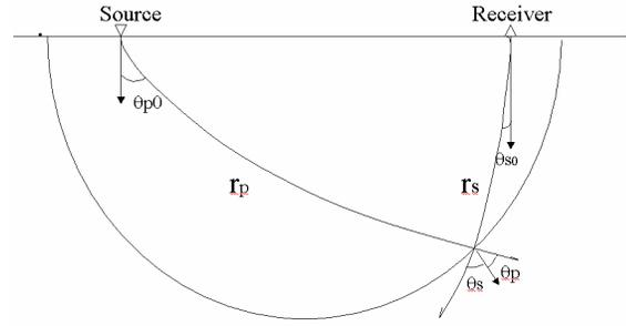
Figure 1, the scattering angles for PS wave.
