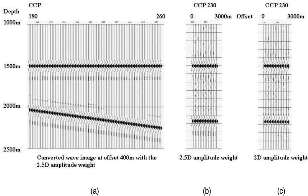
Figure 3. Amplitude comparison for 2D and 2.5D converted wave migration weight functions. (a) 2.5D weight migrated section at offset 400m with two event, one flat and one with 15 degree dip, (b) common image gather at ccp 230 using 2.5D amplitude weight, (c) common image gather at ccp 230 using 2D amplitude weight.
