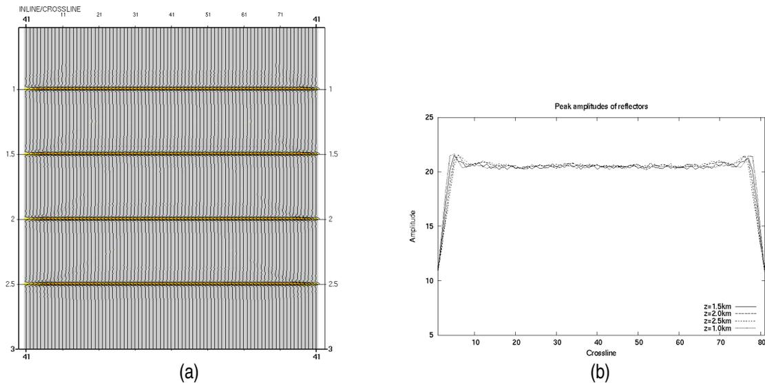
Figure 2. (a) Converted wave migrated section of a 3D synthetic model with four reflections at depths of 1.0, 1.5, 2.0 and 2.5km, (b) the peak amplitudes picked from the four reflections in the left section.
