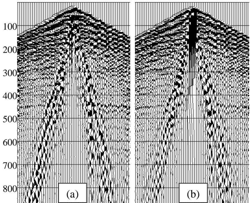
**Figure 1.** Prestack data comparison: (a) shot profile of DSU3 data. (b) VectorSeis® data of the same shot location. The full scale of MEMS (a) is about twice that of MEMS (b) and its recovery time from overdrive is much faster. As a result, overdrive is more apparent on (b).
