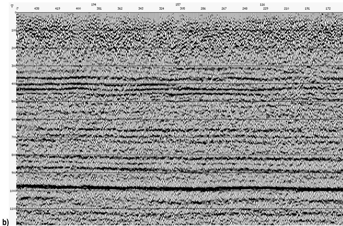
**Figure 3.** Radial data stacked with PS velocity. (a) DSU3. (b) VectorSeis®.
