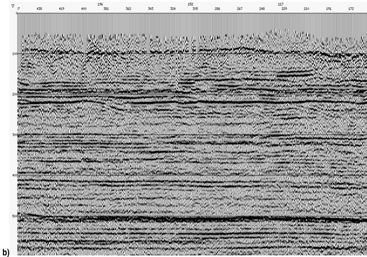
**Figure 2.** Vertical data stacked with PP velocity. (a) DSU3. (b) VectorSeis®.
