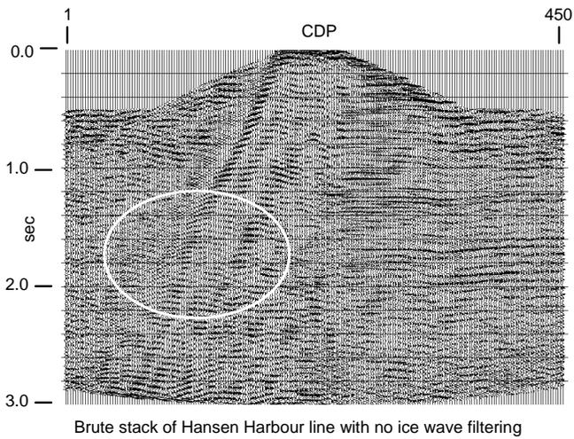
Fig. 9. Brute stack of the vertical component of the Hansen Harbour 3-C experimental line—no coherent noise attenuation.
