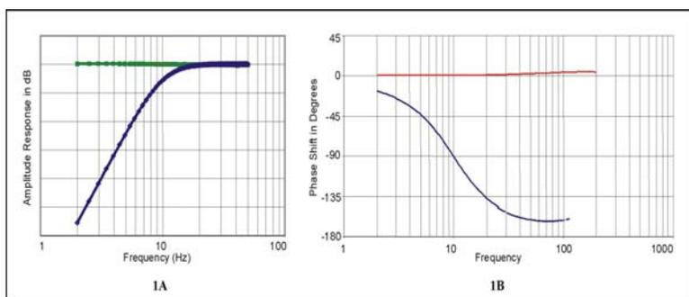
The dark curve in 1a is the amplitude response for the geophone showing a drop-off of amplitude below the natural resonance frequency and the light curve showing the flat response for VectorSeis. Figure 1b shows the impulse response for the geophone (dark line) and the flat phase response for VectorSeis.
