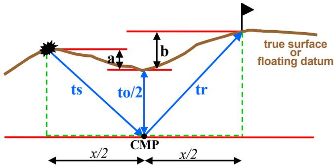
**Figure 2.** Schematic illustration for the derivation of NMO with the double square root equation. 'ts' is the travel time from shot to CMP, 'tr' is the travel time from CMP to receiver, 'to' the two-way zero offset time, and 'x' the source-receiver offset.
