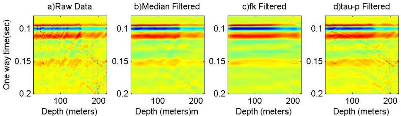
Figure 2. a) Raw VSP data. b) 6 point median filtered data. c) FK filtered data d) t-p filtered data.
