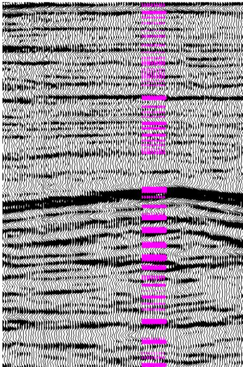
Fig 6 : Correlation of corridor stack (median filtering) with seismic
