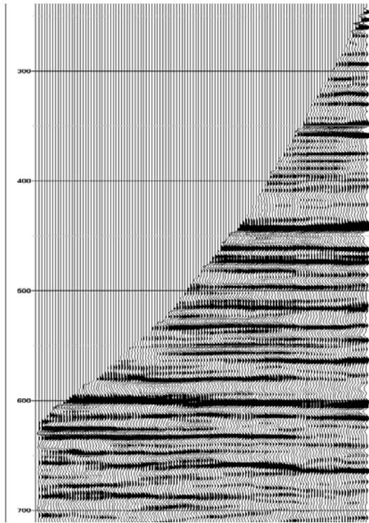
Fig.5 : Aligned upgoing VSP wavefield separated using LIFT
