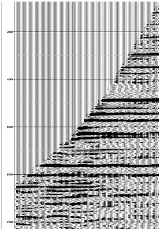
Fig.1 : Aligned upgoing VSP wavefield separated using median filtering
