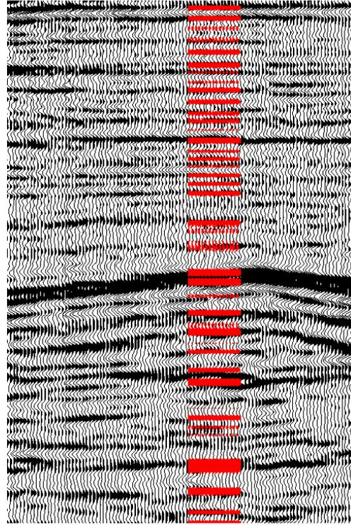
Fig.9 : Correlation of corridor stack (LIFT) with seismic
