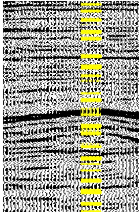
Fig.7 : Correlation of corridor stack (f-k filtering) with seismic
