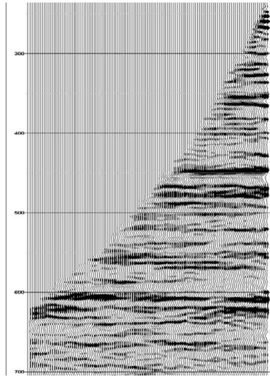
Fig.2 : Aligned upgoing VSP wavefield separated using f-k filtering
