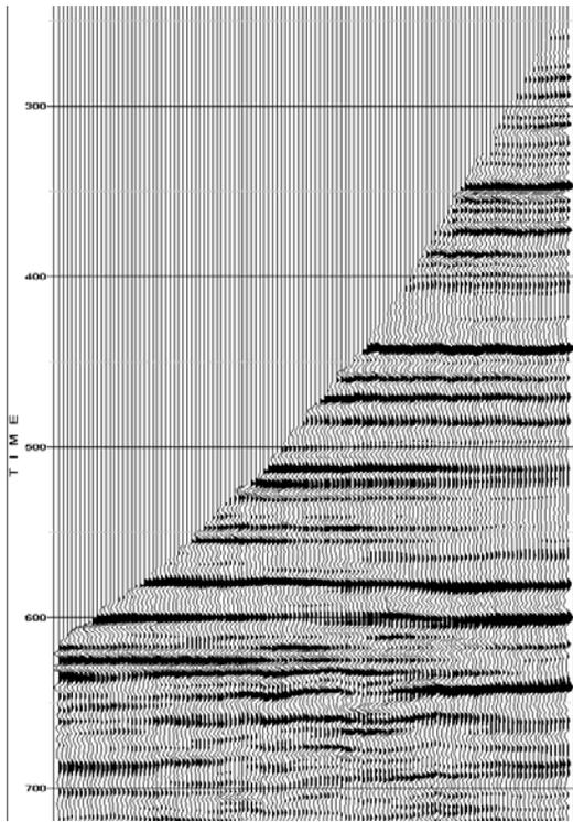
Fig.4 : Aligned upgoing VSP wavefield separated using optimization inversion
