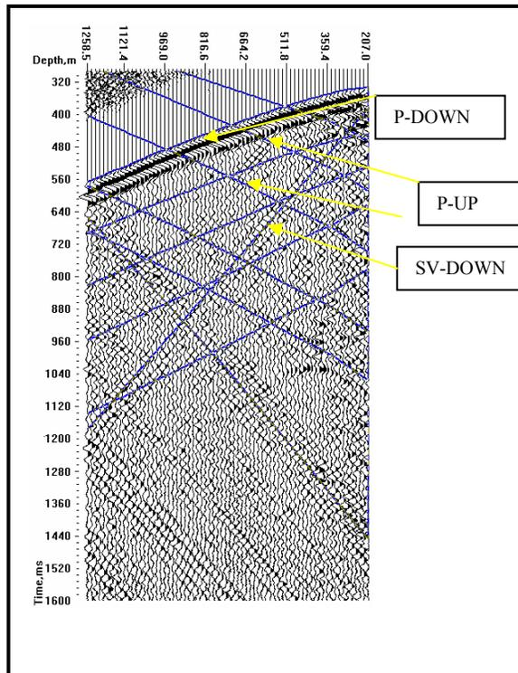
Figure 3: Description of wavefields on a VSP record
