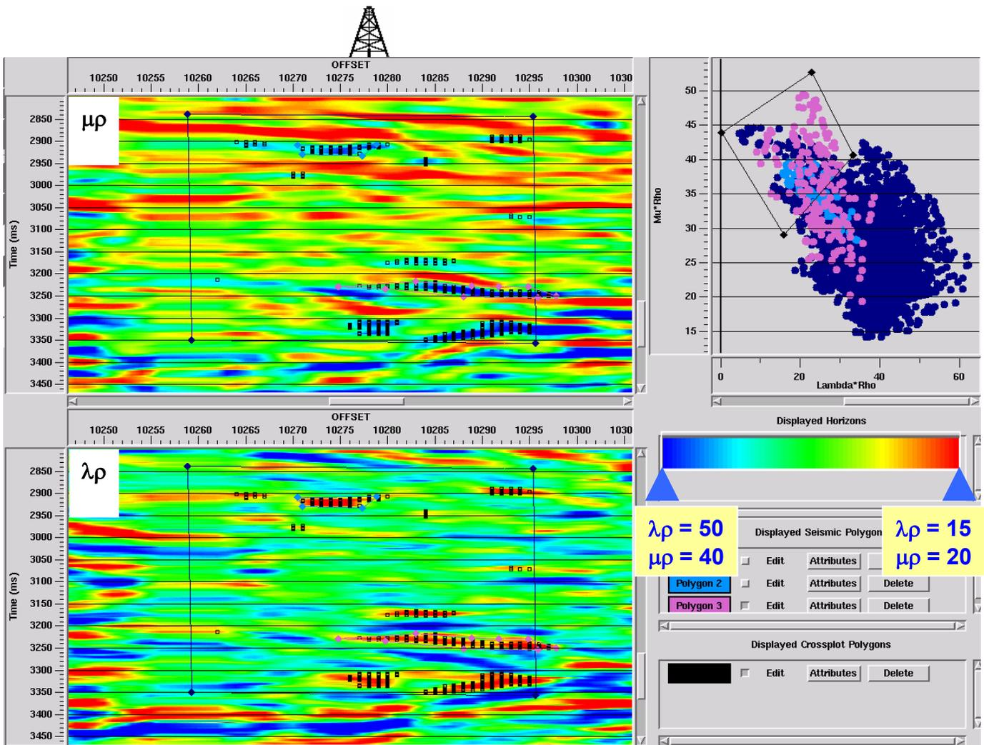
Figure 6: Lambda-Rho and Mu-Rho sections along with the associated cross-plot. A polygon on the crossplot lights up the prospective zones on the two sections.
