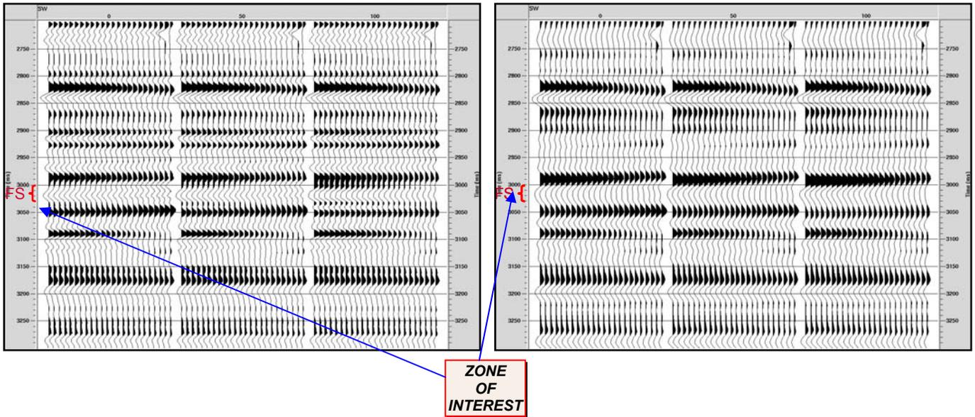
Figure 4: Synthetic gathers generated with a (a) 60 Hz wavelet and (b) 35 Hz wavelet and indicated values of water saturation. Evidently, gathers with 60 Hz exhibit amplitude variation with offset.
