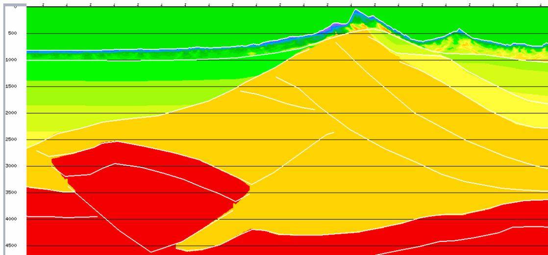
Figure 2: Initial model combining the near surface velocity model and structural interpretation.
