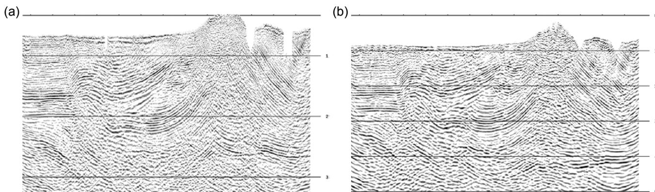
Figure 4. (a) Prestack time migration and (b) Prestack anisotropic depth migration of one of the lines from this project area.
