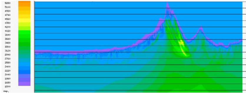
Figure 1: Near-surface velocity model from first-arrival tomography (pseudo-datum not shown)
