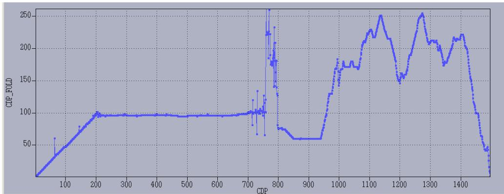
Figure 3: Fold variation along a merged output line.
