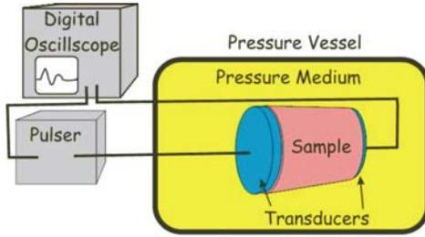
Figure 1: Cartoon of the experimental setup of the velocity measurement.
