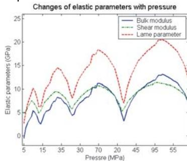
Figure 5: Changes of elastic parameters ( $K_d$ ,  $\mu_d$  and  $\lambda_d$ ) with confining pressure.
