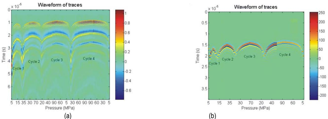
Figure 2: Images of the (a) P-wave traces and (b) S-wave traces under cyclical loading at different confining pressures. The confining pressure is cycled four times from atmospheric to a peak pressure that progressively increases with each cycle
