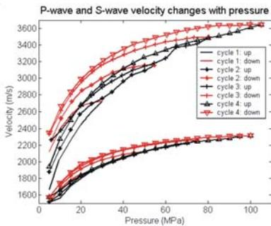
Figure 4: The P- and S-wave velocity changes with confining pressure. The P-wave is measured first, so the sandstone was compacted when the S-wave measurement is taken.
