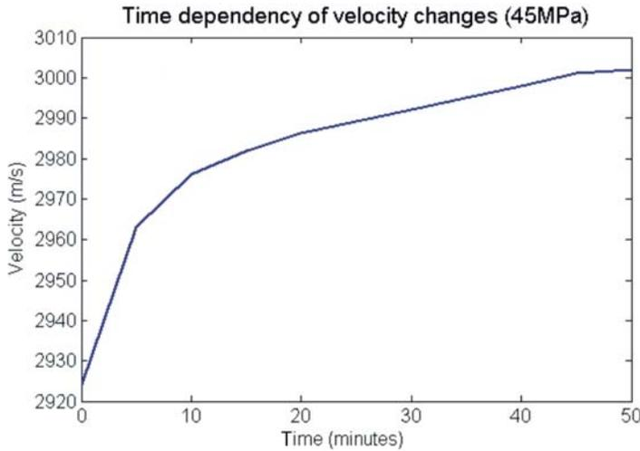
Figure 3: Change in observed  $V_p$  with time at constant confining pressure of 45 MPa
