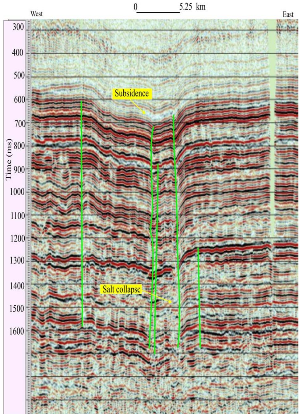
**Figure 2. Effect of a salt collapse on seismic events (Line NOR-83341). Note that this collapse must have occurred more recently than in Figure 1, with all of the overlying strata disturbed by it.**
