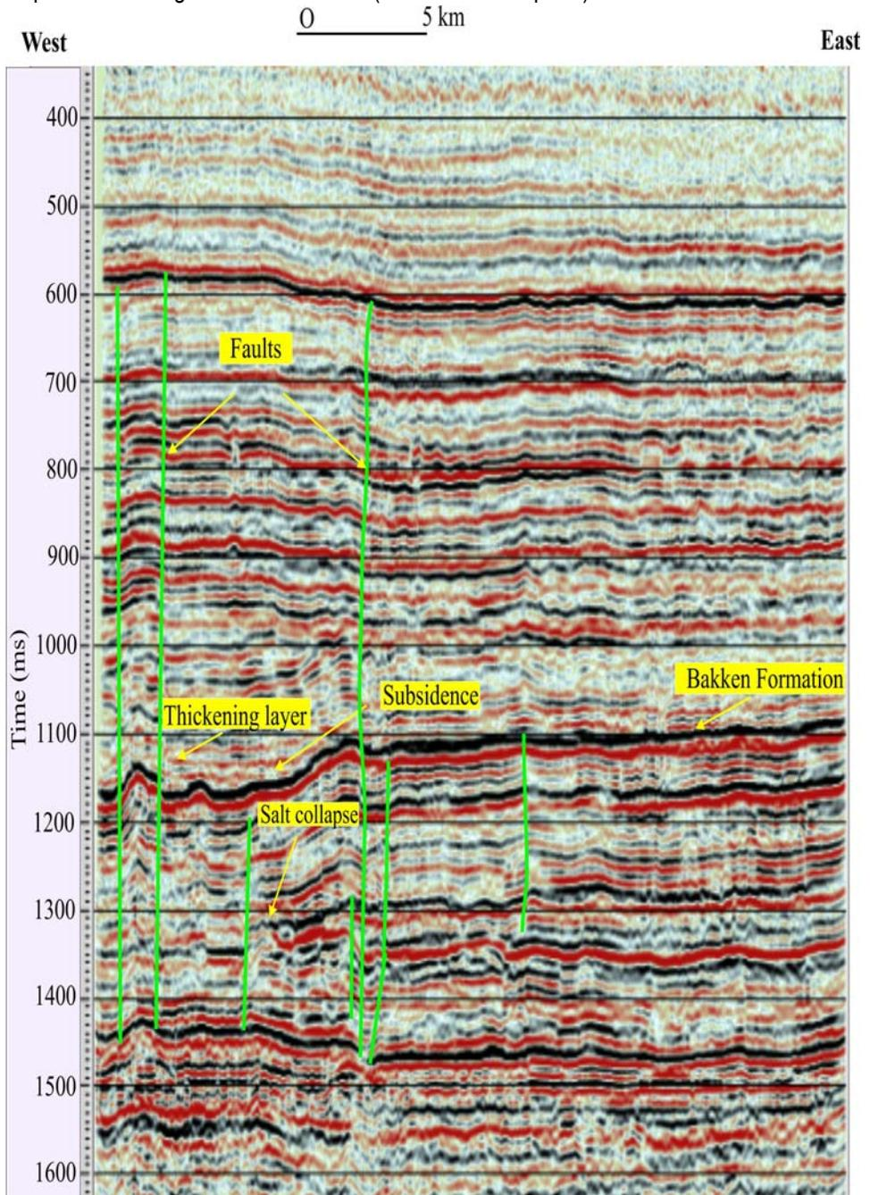
**Figure 1. Subsidence caused by the salt collapse does not affect the shallower strata (Line CBY-5)**
