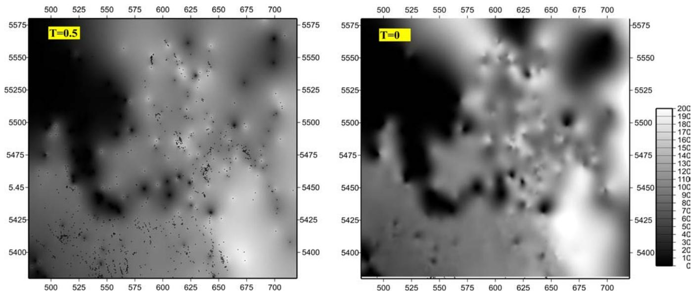
**Figure 3. Prairie salt maps interpolated using GMT programs (Smith and Wessel, 1990), using two values of spline tension parameter  $T$ , as labelled.  $T$  typically varies from 0 to 1, with larger values corresponding to smoother interpolations. Note the differences between maps using different interpolation parameters. Coordinates are UTM in km, black dots in the plot on the left indicate the wells used for interpolation.**
