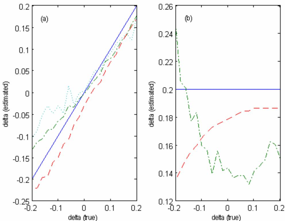
Figure 2. Reflection-traveltime inversion for anisotropic parameters. The crossplots of (a) estimated  $\delta$  vs true  $\delta$ ; and (b) estimated  $\varepsilon$  vs true  $\delta$ . Solid line: the exact anisotropic parameters; dotted line: hyperbolic traveltimes inversion; dash-dot line: three-term Taylor-series inversion; dashed line: nonhyperbolic inversion.
