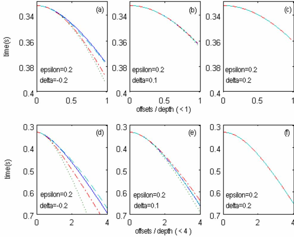
Figure 1. Reflection-traveltime approximation to the true reflection traveltime over a short spread (upper panel) and a long spread (lower panel). Solid line: the exact traveltime; dotted line: hyperbolic traveltime approximation; dash-dot line: three-term Taylor-series approximation; dashed line: nonhyperbolic approximation.
