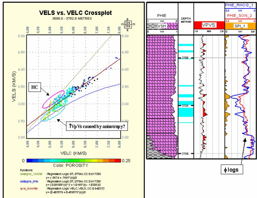
Figure 8: Secondary Porosity Indicator
