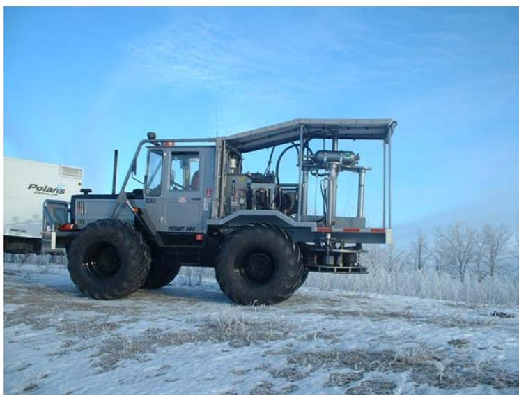
Figure 1: Surface weight drop unit.
