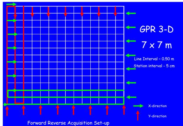
FIG. 2 Acquisition layout of the 3-D grids.
