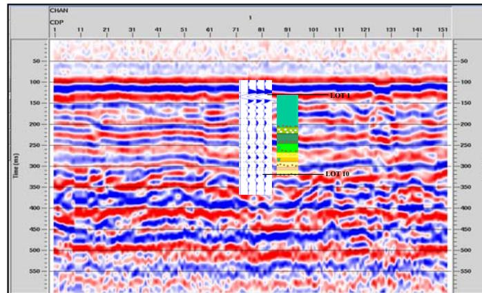
FIG. 4 Comparison of a line from the 3-D grid with radargram.
