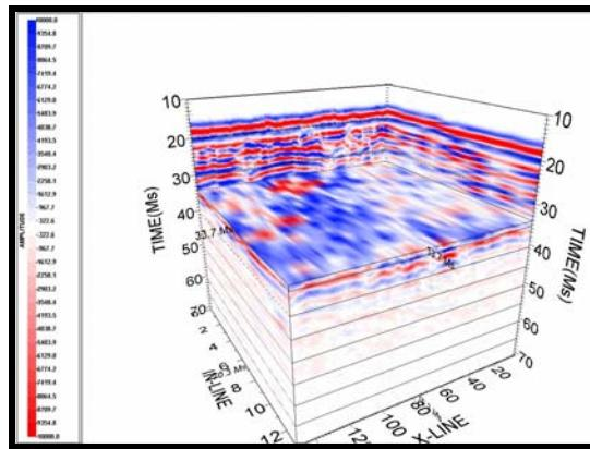
FIG. 6 3-D grid from the X-direction or inline direction.
