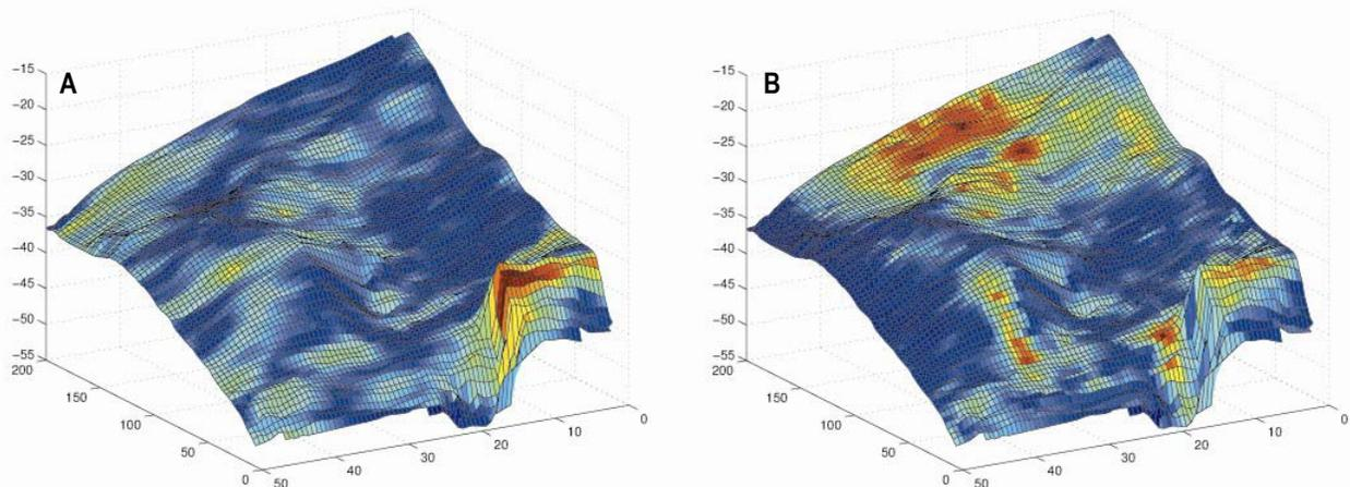
Figure 3. 1984-1999 difference projected onto the Top Ula horizon from ordinary difference cube (A) and computed using Curvelet domain adaptive subtraction (B)
