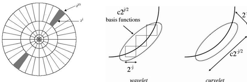
Figure 1. **Left:** Curvelet Partitioning of the Frequency Plane [modified from 3] **Right:** Comparison of non-linear approximation rates for Curvelets and Wavelets [modified from 6]
