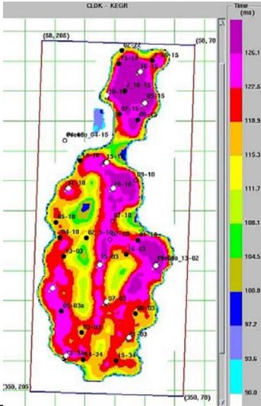
Figure 1. Isochron map from Keg River to Cold Lake; injection wells in white
