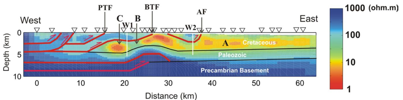
Figure 4 Electrical resistivity model obtained by inversion of the MT data. The structural interpretation is modified from Lagenberg and Kubll (2002); Triangles denote MT stations; PTF=Pineneedle Thrust Fault; BTF=Brazeau Thrust Fault; AF=Ancona Fault; W1=well:100051303712w500; W2=well: 100101603710w500.
