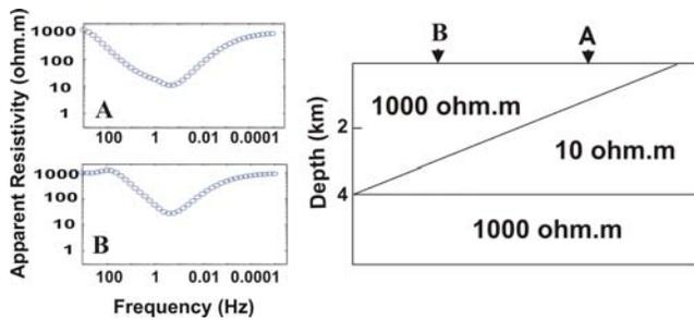
Figure 1: Synthetic model illustrating how MT data can detect a conductive layer. At both stations, the decrease in apparent resistivity is due to the underthrust layer.
