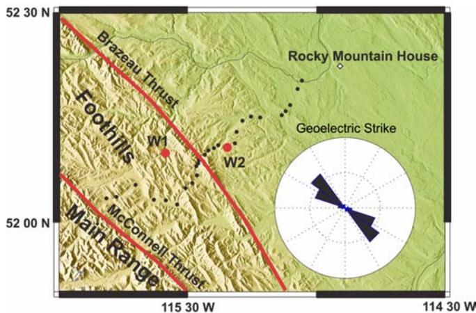
Figure 3: Location map of the MT stations in Rocky Mountain Foothills (squares). The rose diagram shows the strike direction determined from the MT data, which agrees with the regional geology. Black dots denote locations of MT sites. Red dots denote well locations.
