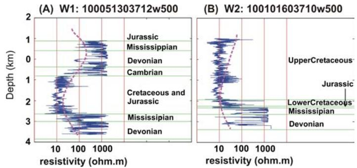
Figure 2: Comparison of resistivity logs (solid lines) and the MT derived resistivity model (dashed lines) at the two well locations shown in Figure 3. Depth is relative to sea level.
