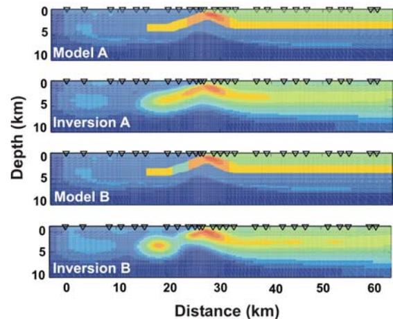
Figure 5: Synthetic inversion study used to test sensitivity of data to the underthrust layer. Synthetic data were computed for both models A and B. The resistive break (B) in Figure 4 is clearly required by the data. Resistivity scale is the same as in Figure 4.
