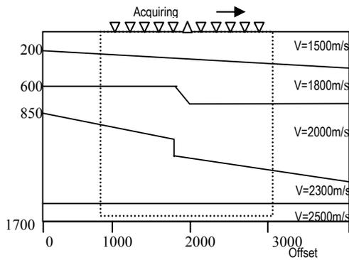
FIG.6. Subsurface model. The dashed line defines the image window. The velocity for each layer is labelled in the model. The transition frequency  $\omega_0$  of this model is 20000.
