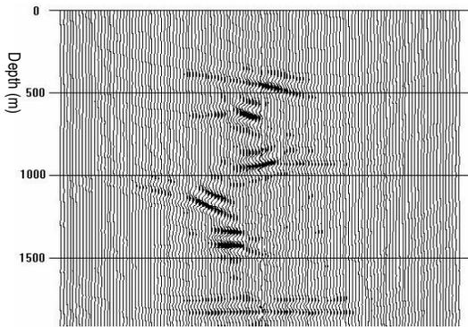
FIG. 8. The images resulting from acoustic wave equation prestack depth migration
