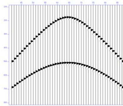
FIG.3. Acoustic forward modelling result from the same geological model of Fig.2 but the attenuation is zero
