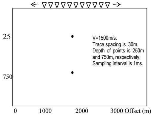
Fig 2. Geological model for forward modeling
