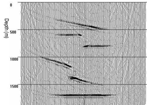
FIG. 9. The images resulting from viscoacoustic wave equation prestack depth migration.
