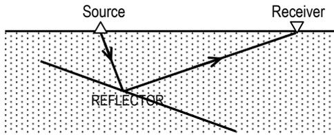
FIG. 1. Raypath of a reflected signal. The wave is compensated for absorption on the way from the source down to the reflector, and up to the receiver.
