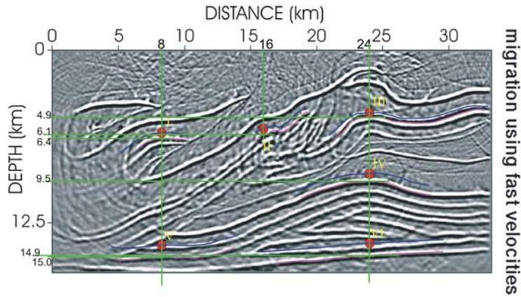
Figure 3 - This section displays a poststack reverse-time depth migration using a 10% fast velocity model. The six features (I, II, III, IV, V, and VI) are now imaged at deeper locations identified with pink horizons. The new depth coordinates are marked on the vertical axis (only noting the vertical displacement). The true features indicated with the red circles and horizons marked in blue have been superimposed on this section, which displays the original features I - VI.
