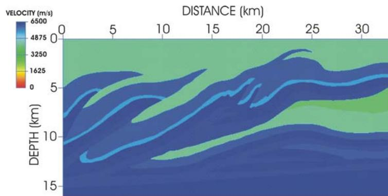
Figure 1 - This shows the true velocity model used for the various depth migrations. Numerous perturbations (10% too slow / fast and random) were applied to this model to test the sensitivity of the depth migrations.
