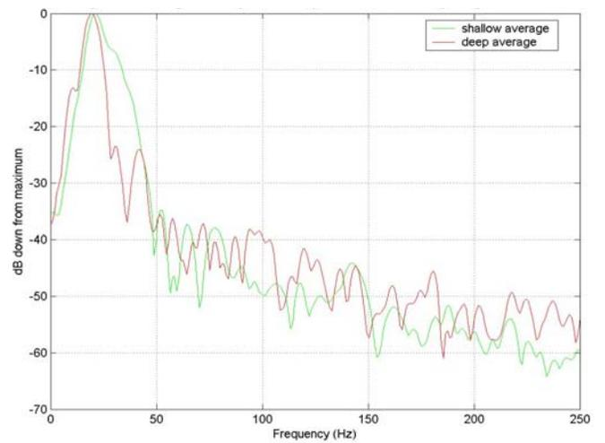
Figure 5. Averaged Amplitude Spectra of S-Wave
