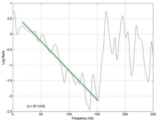
Figure 3. Spectral Ratio Plot of Downgoing P-Wave
