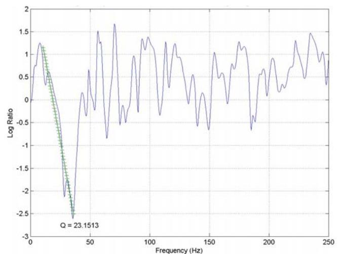
Figure 6. Spectral Ratio Plot of Downgoing S-Wave
