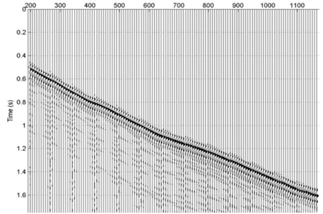
Figure 4. Downgoing S-Wave (depth(m) vs. time(s))
