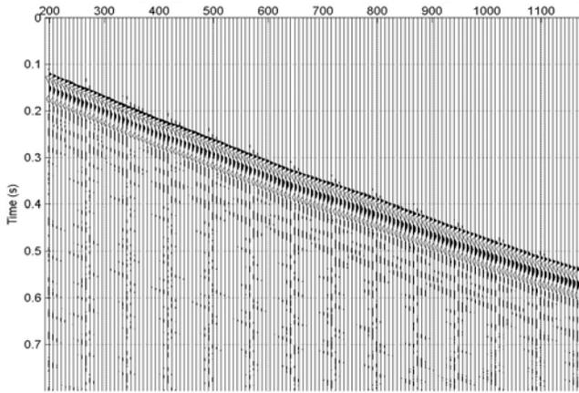
Figure 1. Downgoing P-Wave (depth(m) vs. time(s))
